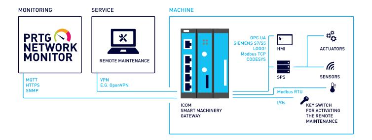
Here you can see that on the one side, the gateway is connected to various aspects of the factory floor, such as actuators, sensors, and other control mechanisms. On the other side, the gateway connects to operators (like ERP or SCADA systems), services and manufacturers.
